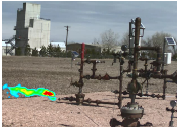
Image: Experiment equipment at Colorado State University, U.S. Plant operation Visualize invisible gases to ensure safety
