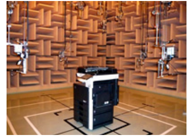
The inside of the acoustic test laboratory
